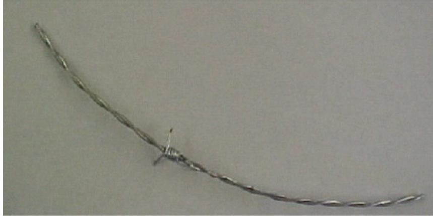
The permissible variation from the nominal diameter of the wire, for both line wires and barbs, for all types, shall be  $\pm 0.005$  inches.
